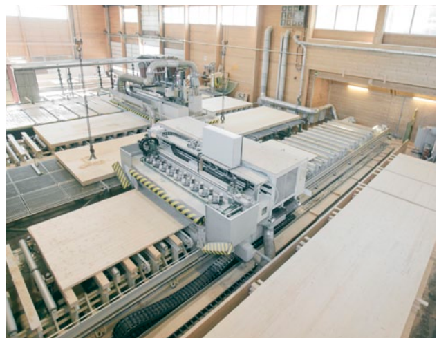
State-of-the-art CNC cutting machines facilitate simple and highly complex cutting patterns
