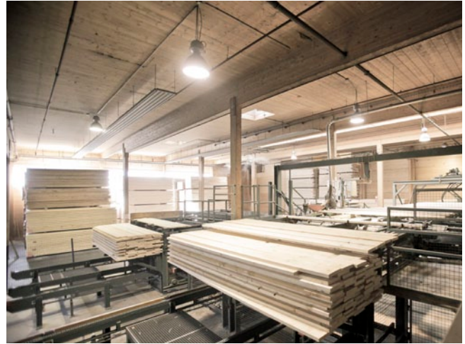
Cross-laminated timber is produced on a just-in-time basis
